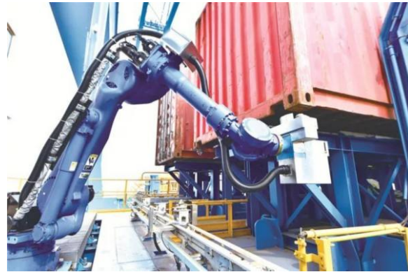
Figure 7. The twist lock handling system developed by Qingdao Port
