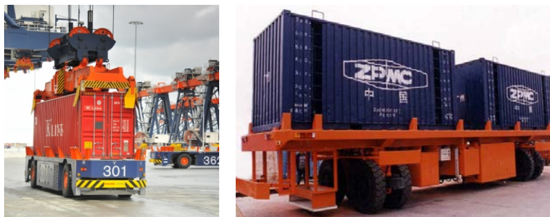
Figure 3. AGVs used in automated container terminal
